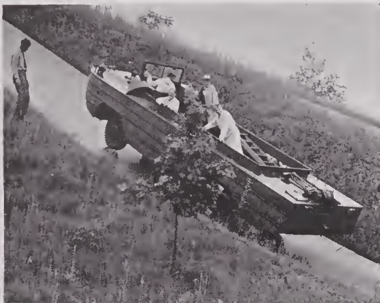
FIGURE 45. First pilot model DUKW climbing 60-degree grade at Milford, Michigan.
